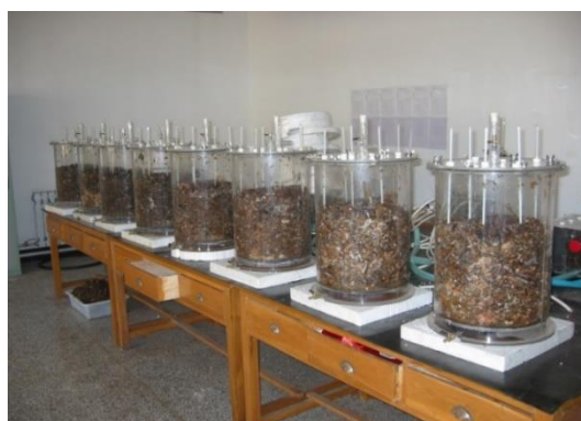
Figure 1. Experimental photo and apparatus used in the aerobic composting with livestock manures
