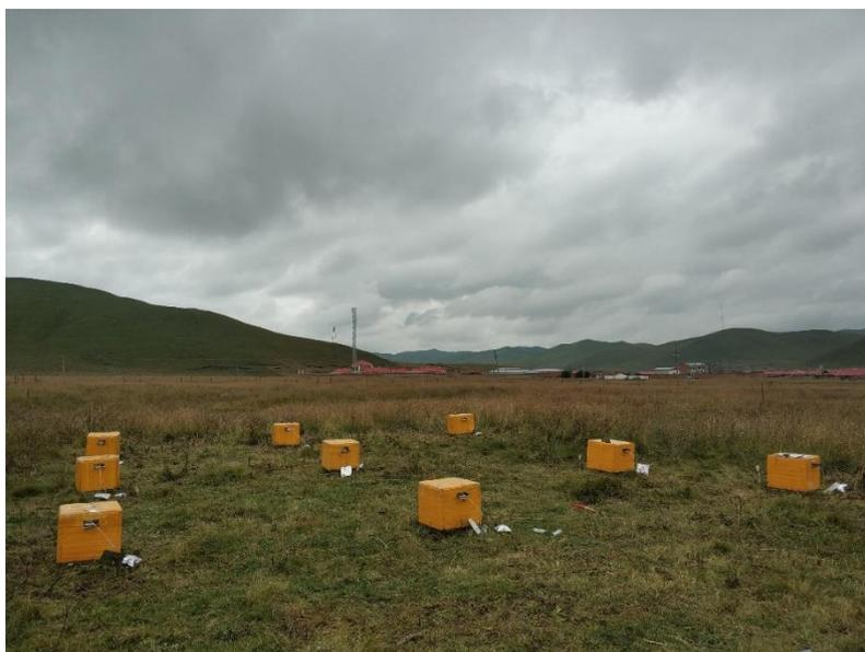
**Figure 2.** Nitrous oxide emissions measurement using static chamber method at Maqu Grassland Agriculture Research Station of Lanzhou University, China
