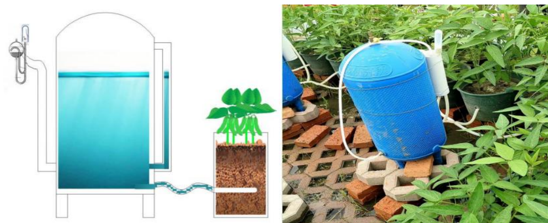
Figure 1. Installation diagram (a) Water outlet: Connects to the clay pipe, controlling water entry into the root zone (b) Water storage bucket: Stores water and maintains its level (c) Negative pressure stabilizer: Ensures a stable water supply by regulating negative pressure (d) Clay pipe: Buried in the root zone, allows water infiltration based on negative pressure
