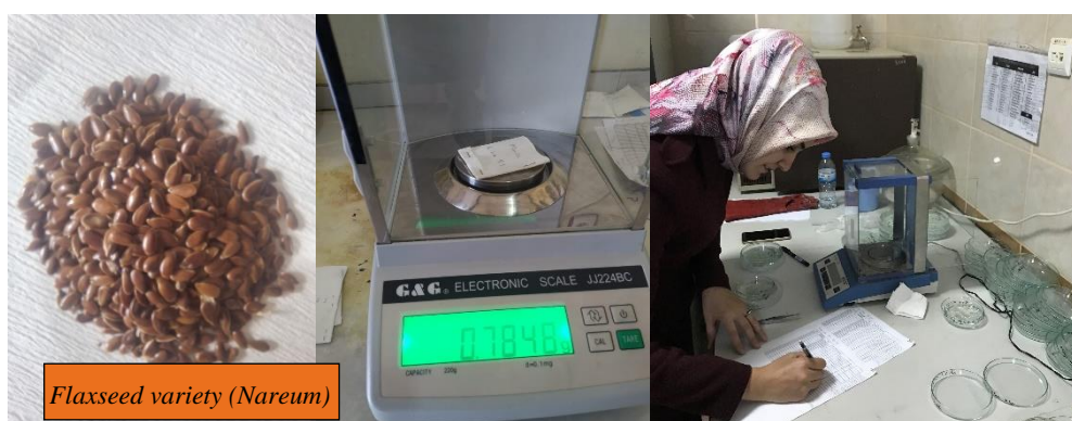
Figure 1. Flaxseed variety (Nareum) used in the experiment (date of supply 27.12.2019), and in the laboratory with climate cabinet, an oven, precision scales, etc., on the 15th day after placing, while seeds are measured for germination, radicle, plumule and seedling development
