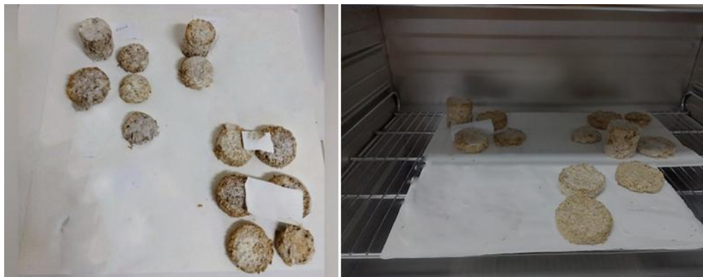
Figure 5. Biomaterials fully developed in the mold and oven-dried
