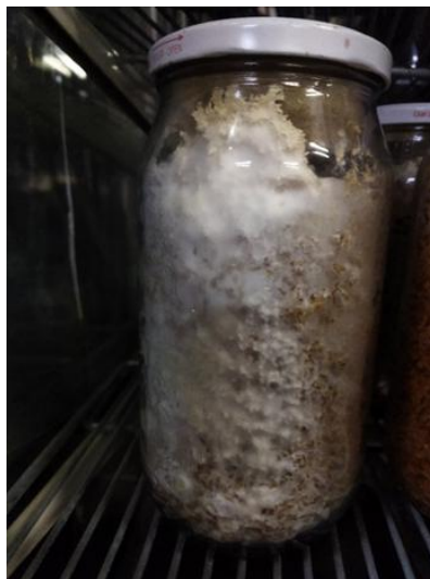
Figure 4. Fully developed mycelium-substrate mixtures in the jar
